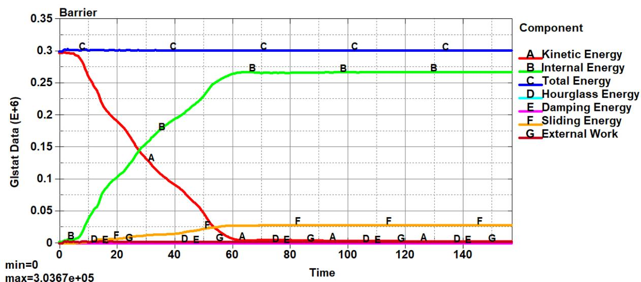
Figure 39: Generic N1 FE model energy balance
