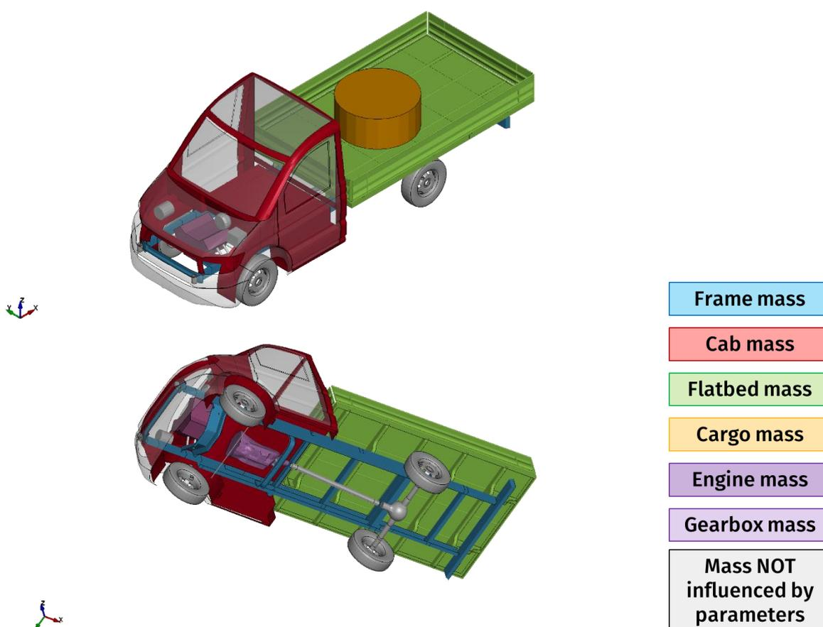
Figure 4: Sets for different mass parameters
