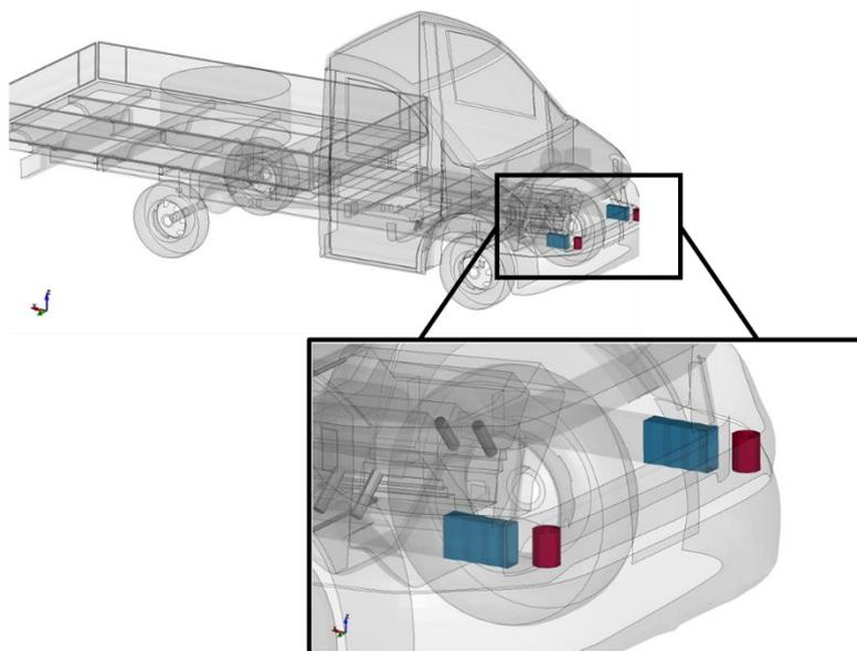
Figure 5: Parts influenced by crash related stiffness parameters
