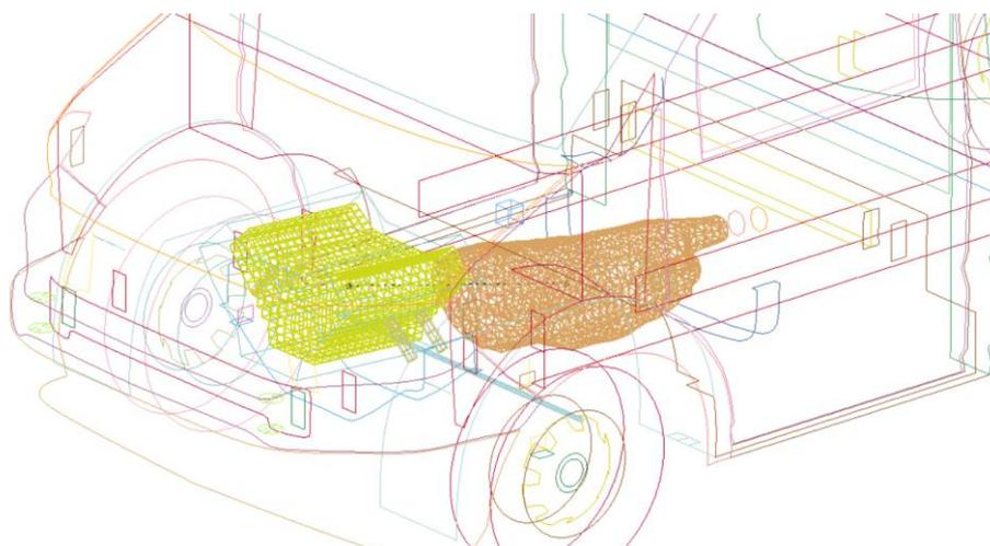
Figure 16: Beam elements connect the engine and the gearbox to the frame
