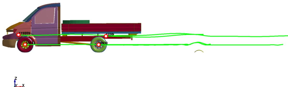
Figure 29: FE vehicle in curb test – trajectories of marked points
