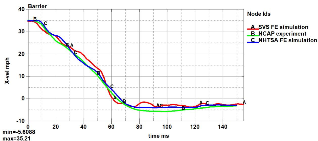
Figure 37: FE models and experiment comparison: Velocity of the vehicle (filter SAE 60Hz)
