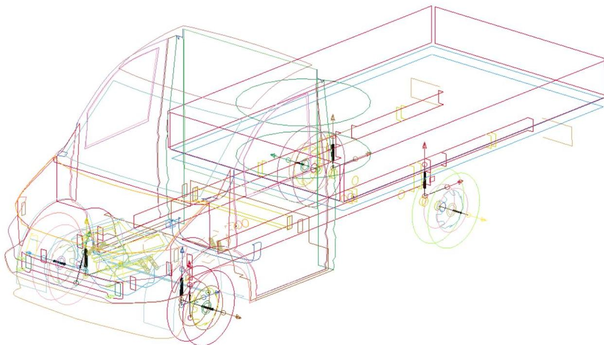
Figure 17: Kinematic joints for wheels
