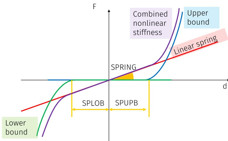
Figure 7: Nonlinear stiffness of suspension
