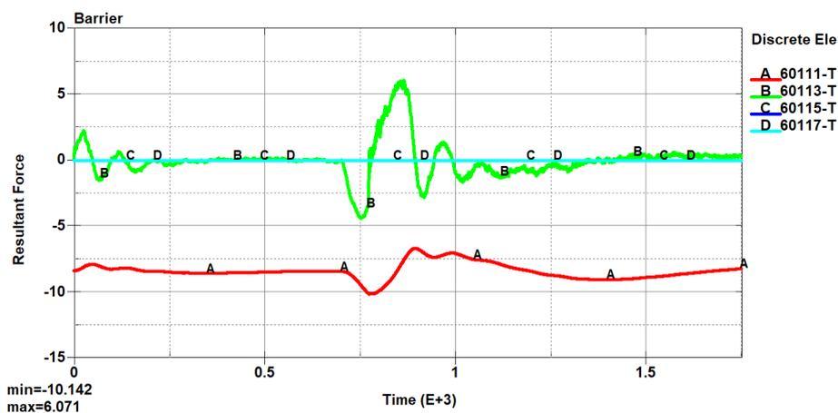
Figure 31: Forces on right rear wheel suspension (A – Linear spring, B – Damper, C – Upper bound, D – Lower bound)
