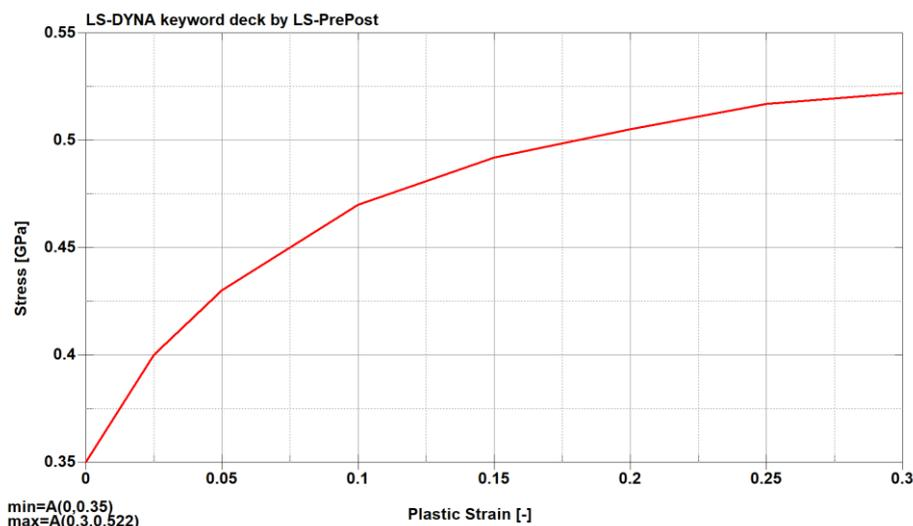
Figure 14: Conventional structural steel #2 plasticity curve
