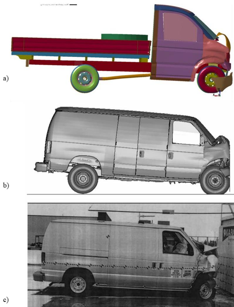
Figure 36: Rigid wall crash test: a) NI generic model, b) Ford Econoline FE crash test by FHWA / NHTSA National Crash Analysis Center, The George Washington University, c) Ford Econoline NCAP test
