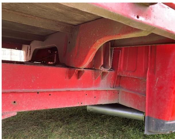
Figure 3: *Main frame of the vehicle and reinforcement of the flatbed*
