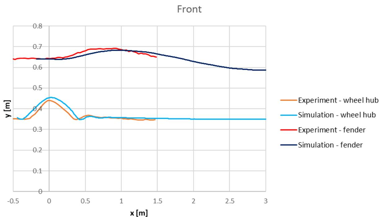
Figure 34: Curb test – sideview trajectory comparison simulation vs experiment – front axle
