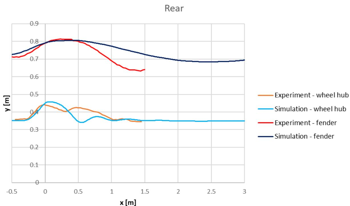
Figure 35: Curb test – sideview trajectory comparison simulation vs experiment – rear axle
