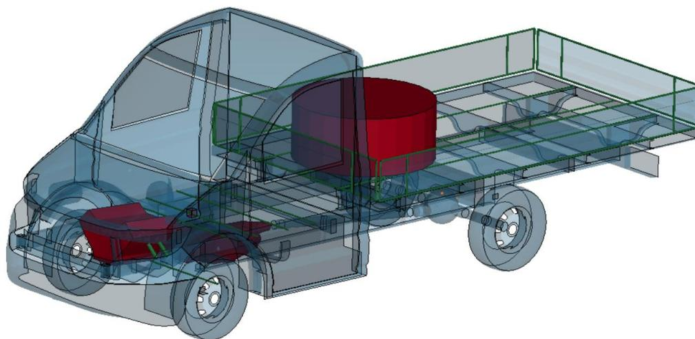
Figure 11: Element types on the vehicle model (solids – red; shells – blue, beams – green)
