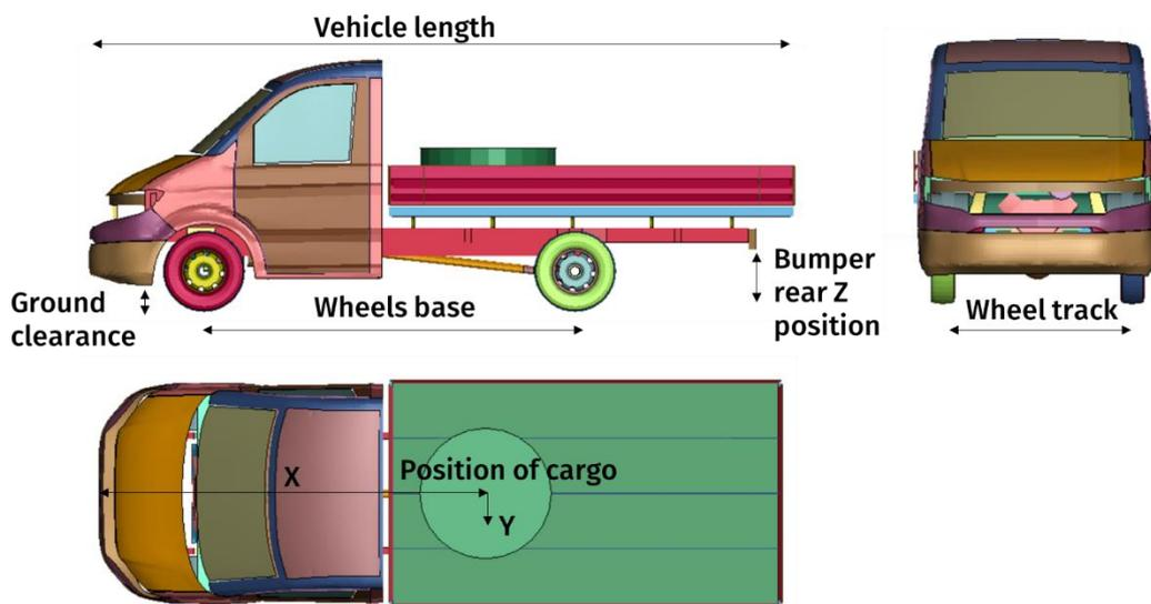
Figure 2: Main parameters of dimensions
