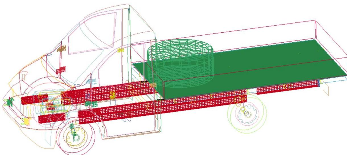
Figure 21: Tied contacts: flatbed – frame and cargo – flatbed
