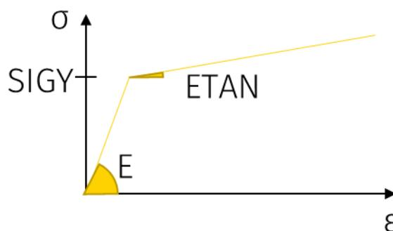
Figure 6: Bilinear elastoplastic behaviour of selected parts governed by crash related stiffness parameters
