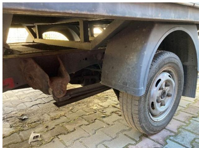
Figure 2: *Rear wheel suspension*
