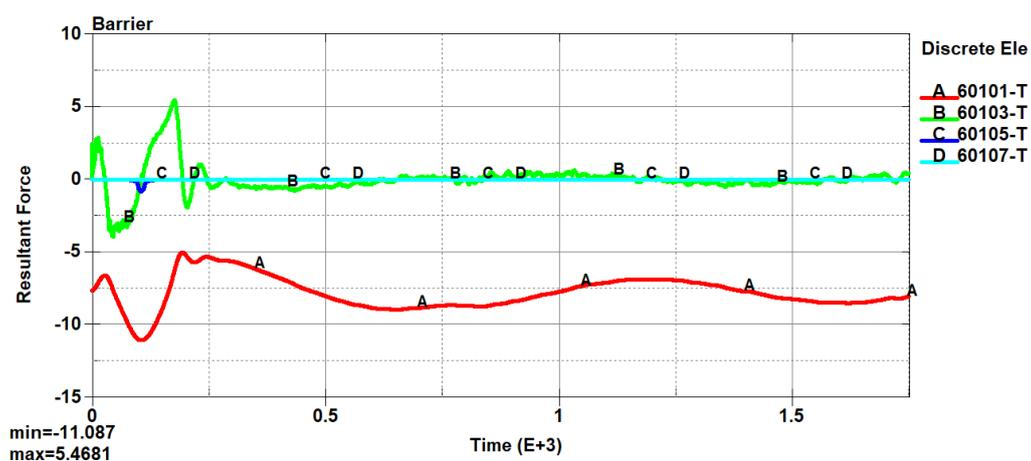
Figure 30: Forces on front wheel suspension (A – Linear spring, B – Damper, C – Upper bound, D – Lower bound)
