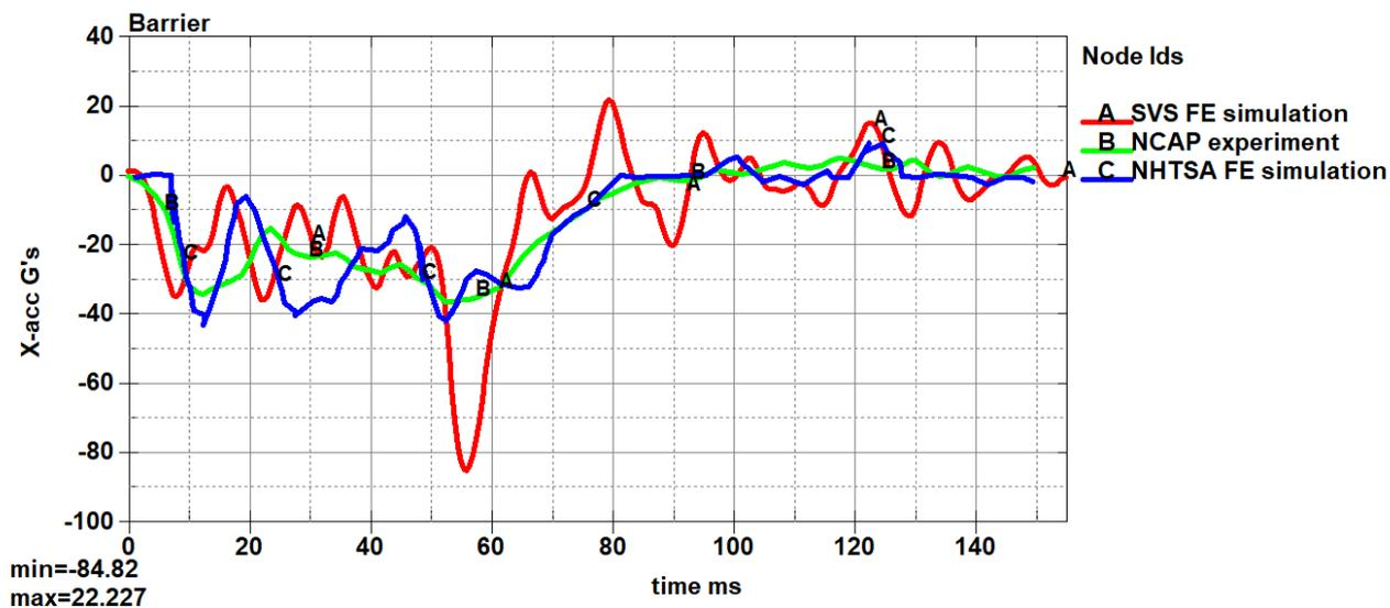
Figure 38: FE models and experiment comparison: Acceleration of the vehicle
