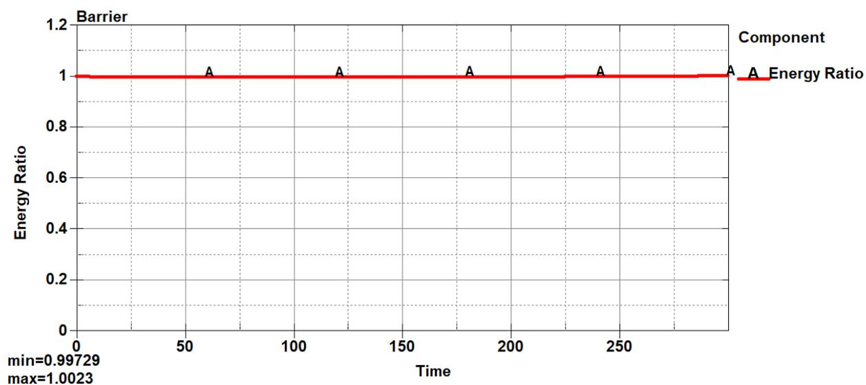
Figure 40: Generic N1 FE model energy ratio
