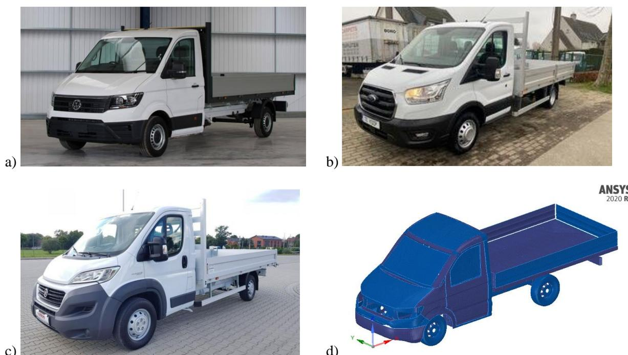
Figure 10: Vehicle geometry: a) VW Crafter, b) Ford Transit, c) Fiat Ducato, d) Generic vehicle geometry
